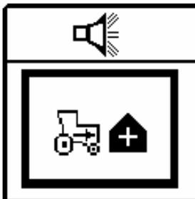
An audible 2-chirp alarm is also output during navigation or data entry to indicate an illegal or non-functional key press.
