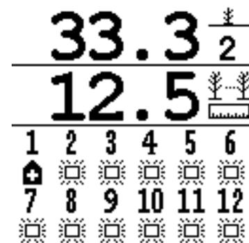
Row scan and average spacing with blinking symbols and row 1 hi alarm (alarm cancel returned user to operate screen)
